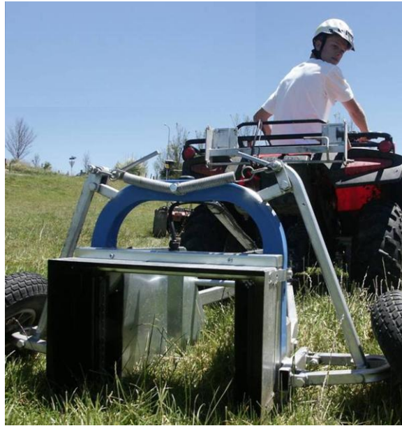
Figure 12 C-Dax pasture meter in operation. (Photo: NZCPA, Massey University).
